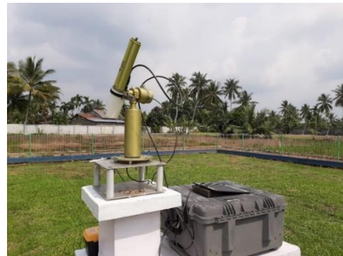
Figure 2. Sun photometer in Mempawah Climatological Station, Pontianak.
