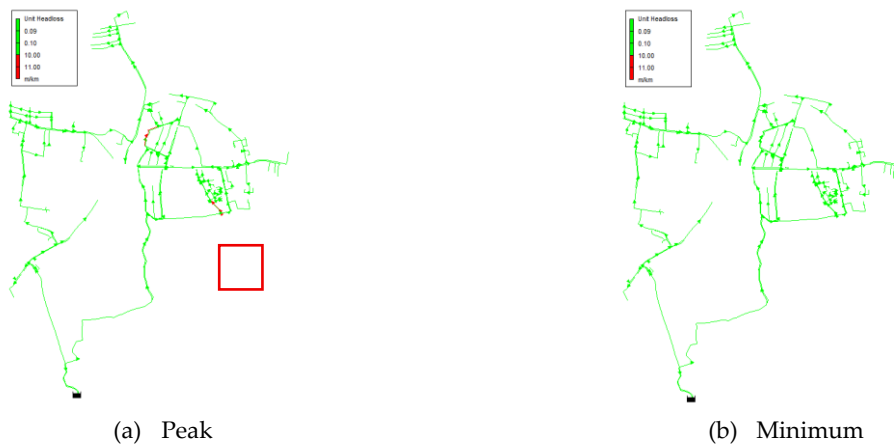
Figure 5. Analysis results of head loss in existing distribution network
