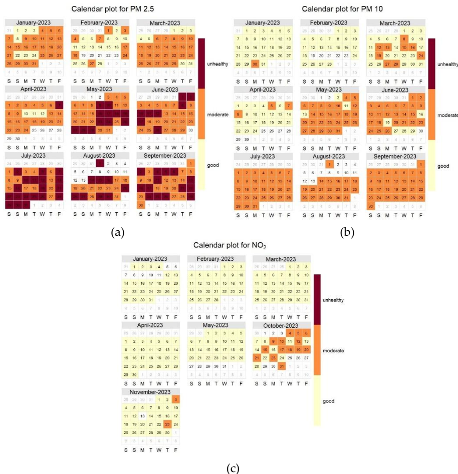
Figure 4. Calendar plot of ISPU (a) PM 2.5 parameter; (b) PM 10 parameter; (c) NO 2 parameter
