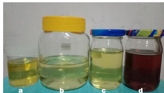
Figure 4. Sample product variants include (a) CME with organic catalysts; (b) CME with KOH inorganic catalyst; (c) PME; and (d) B0.
