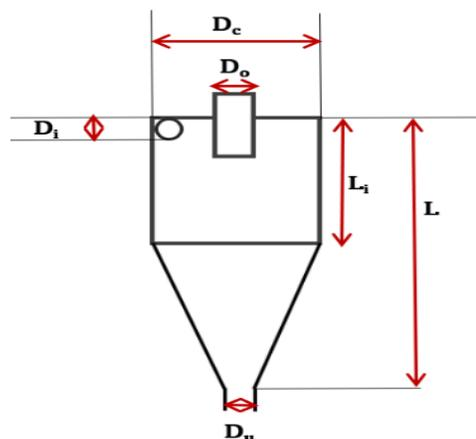
**Figure 3.** Hydrocyclone Geometric Dimensions. Generally, the geometric ratios are determined by either Rietema or Bradley design
