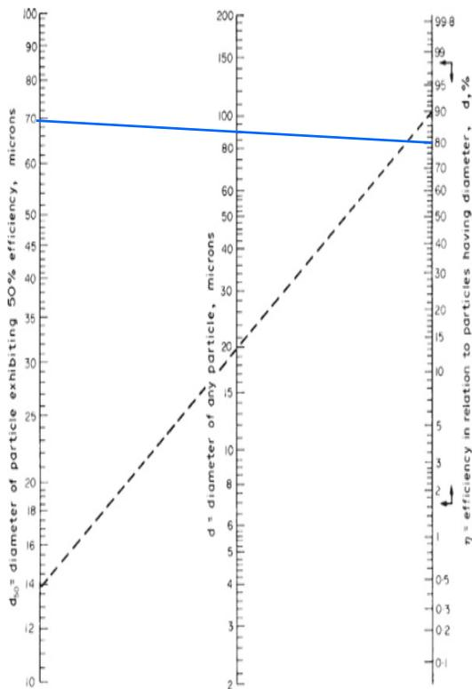
**Figure 5.** Zanker Nomograph for  $D_{min}$  Estimation.
