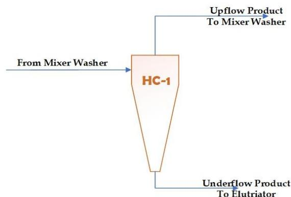
**Figure 2.** Block Diagram of Hydrocyclone in Industrial Grade Salt Pilot Plant Capacities 40,000 TPY in Manyar, Gresik, East Java.
