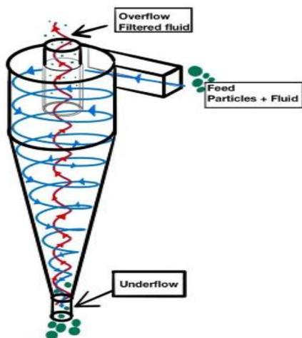
**Figure 1.** Hydrocyclone Schematic Process Flow. [8]
