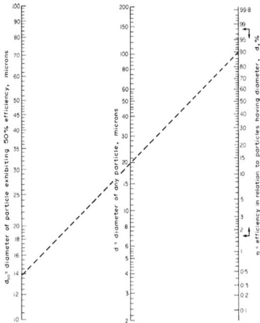
**Figure 4.** Zanker Nomograph. [12]
