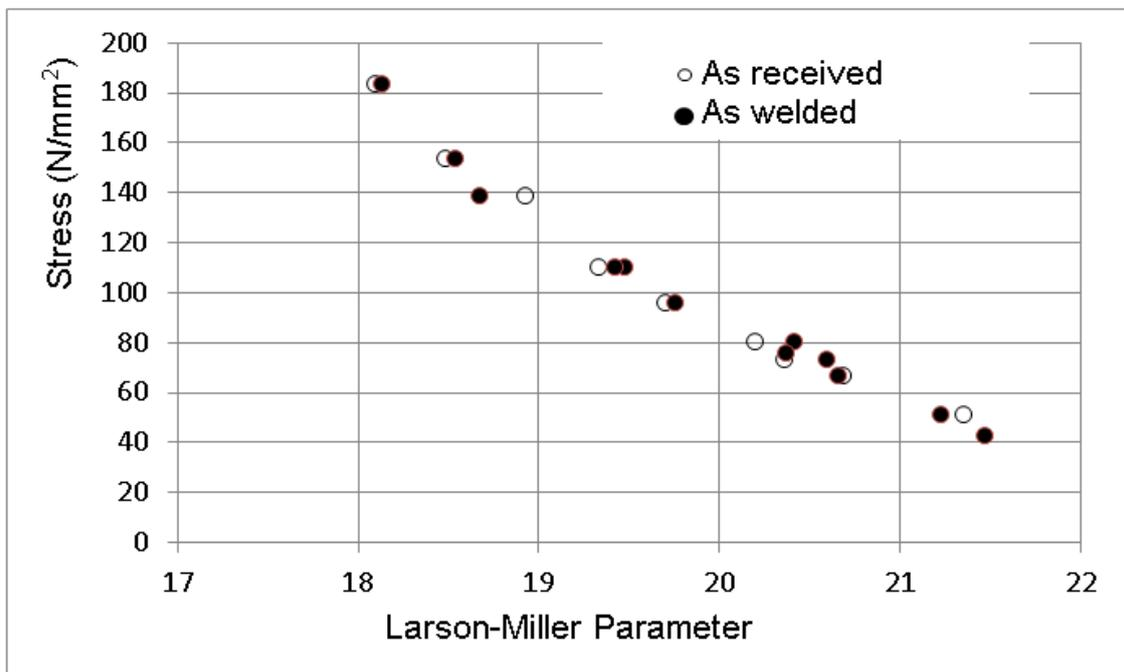
Figure 8. LMP curve of the as-received and as-welded specimen.
