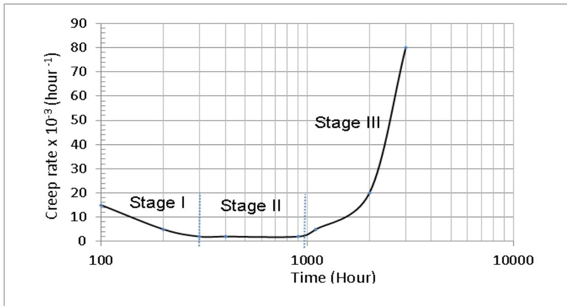
Figure 4. Creep rate curve obtained from creep curve (Using the same data as shown in figure 3).
