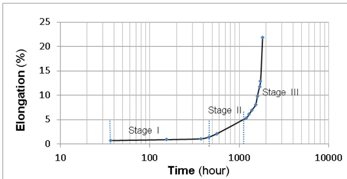
Figure 3. Representative creep curve, the data taken from D-3 specimen (650°C, 43.13 N/mm<sup>2</sup>) with 43.13 N/mm<sup>2</sup> of stress and 650°C of temperature.
