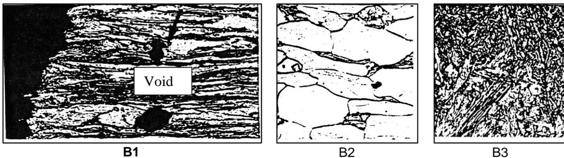
**Figure 5b.** Metallography of the specimen, (B) as-welded specimen.
