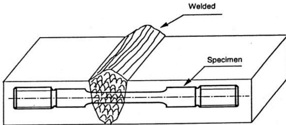
Figure 2 . Welded position on the specimen.
