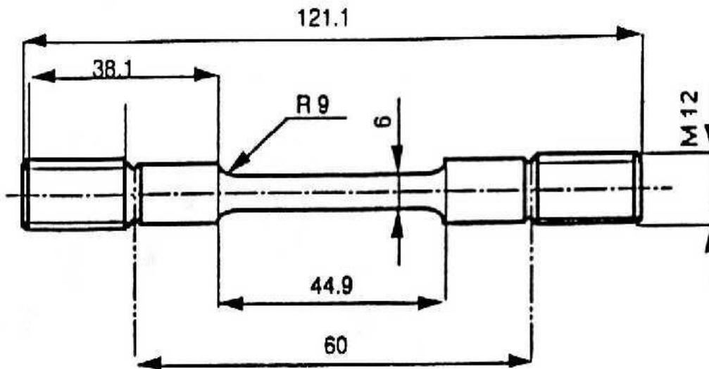
**Figure 1 .** Dimension of the specimen (mm).
