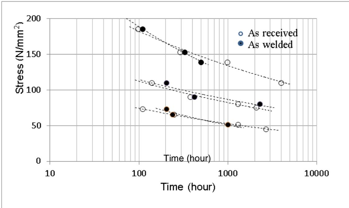
Figure 7. Stress Rupture Curve.
