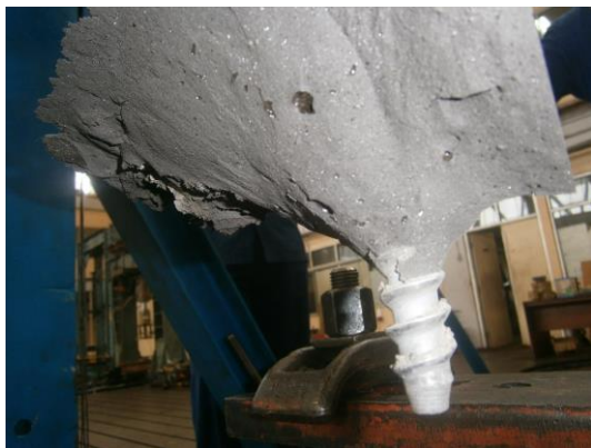
Gambar 8. Model Kerusakan Screw Spike
