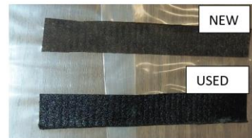
Figure 5. Visual appearance of new and used water separator filters.
