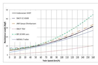
Figure 1 Comparison of Resistance Loads for various Trains
