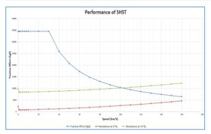
Figure 4 Tractive Force and Resistance Forces as function of Train speed
