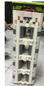
Figure 3. Li-On Battery without case
