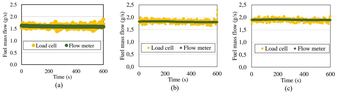
Figure 5. Mass flow rate measurement comparison at (a) 1500 rpm, (b) 1900 rpm, and (c) 2200 rpm
