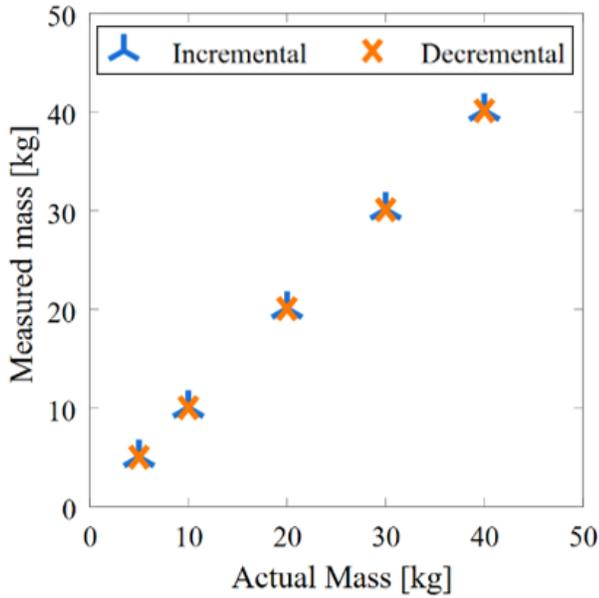
Figure 3. Load cell Calibration Results
