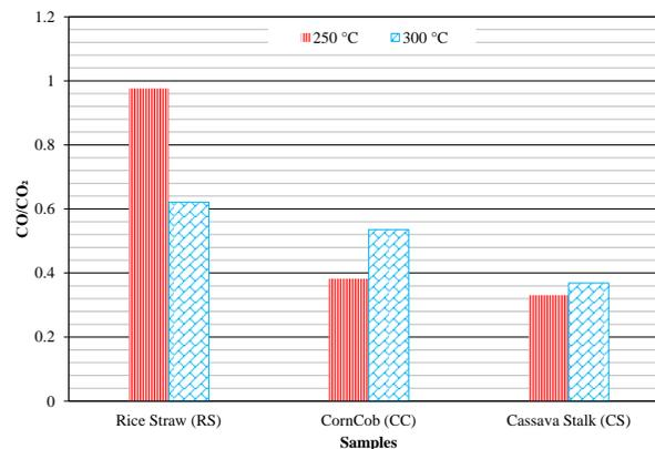
**Figure 7.** Carbon ratio of samples after torrefaction.
