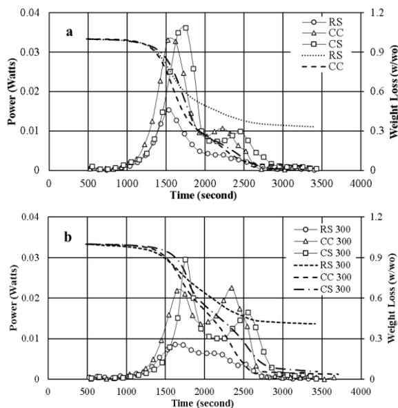
**Figure 6.** DTG curve of combustion Process: (a) raw agricultural crop residues & (b) Torrefied raw agricultural crop residues.
