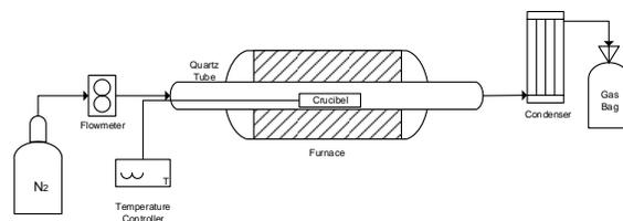
**Figure 3.** Schematic Diagram of the Static Tubular Reactor.
