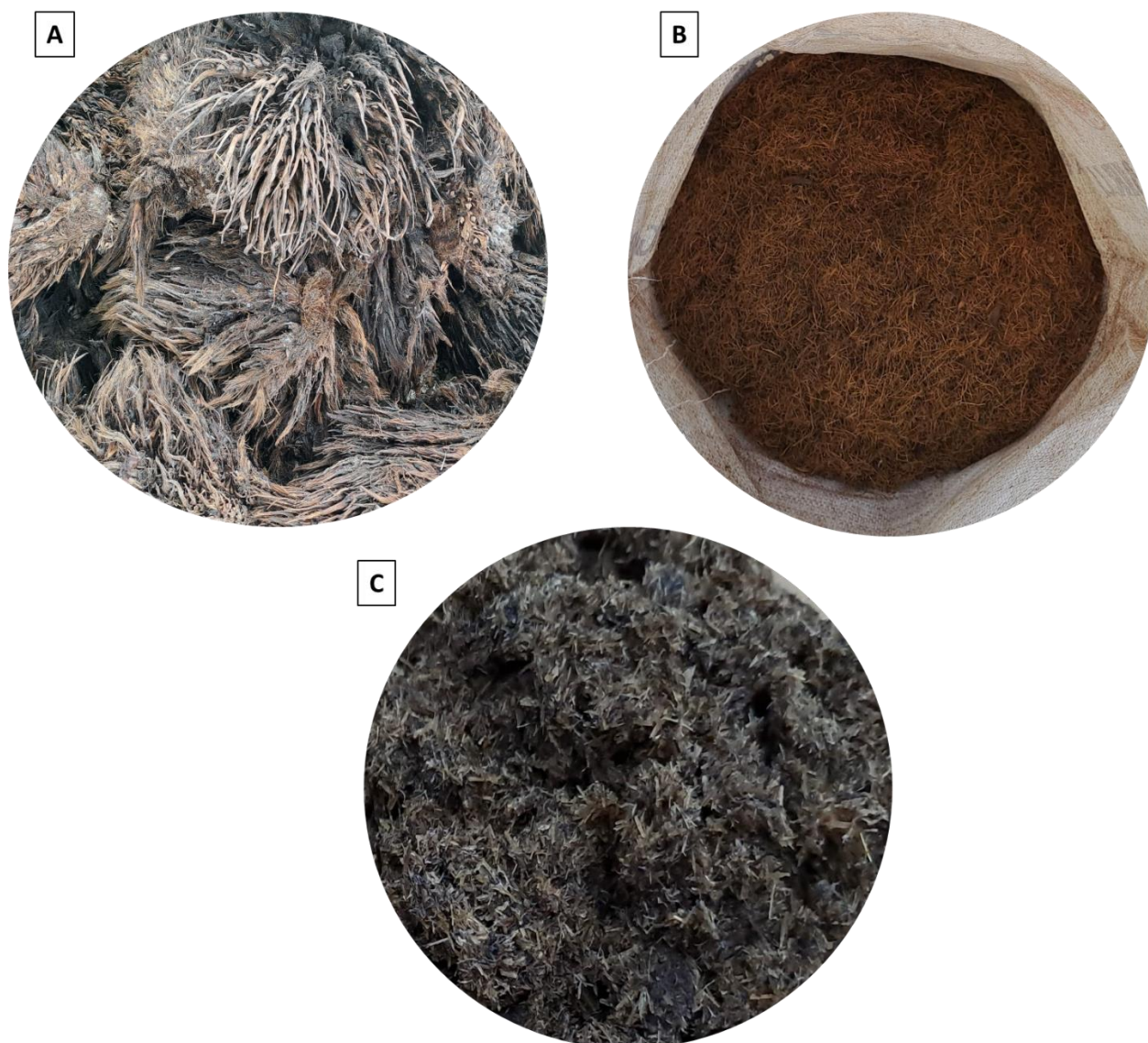
Figure 2. (a) raw OPEFB, (b) OPEFB after physic treatment, and (c) Chemical pretreated OPEFB
