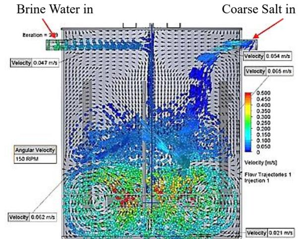
Fig. 3. Velocity Flow Contour projection blade rotation 150 rpm
