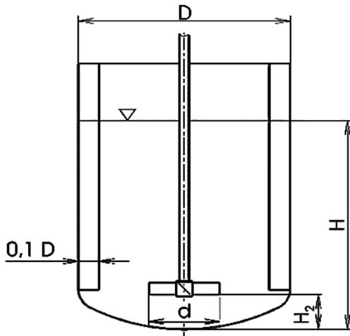
Fig. 2. Standard Mixing Tank
