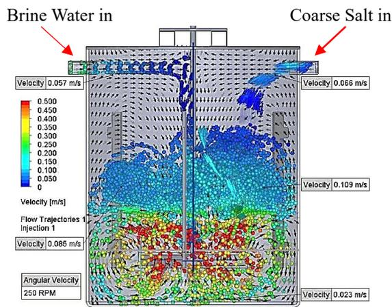
Fig. 5. Velocity Flow Contour projection blade rotation 250 rpm
