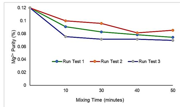
Fig. 8. Relationship between processing time in the mixing washer and Mg<sup>2+</sup> impurity across three run tests.
