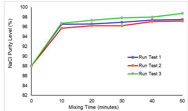
Fig. 7. Relationship between processing time in the mixing washer and NaCl purity across three run tests.
