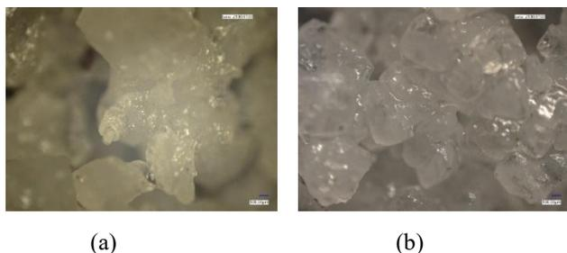
Fig. 9. Visualization with 100x magnification of coarse salt (a) and washed salt (b)
