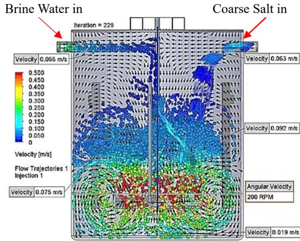
Fig. 4. Velocity Flow Contour projection blade rotation 200 rpm
