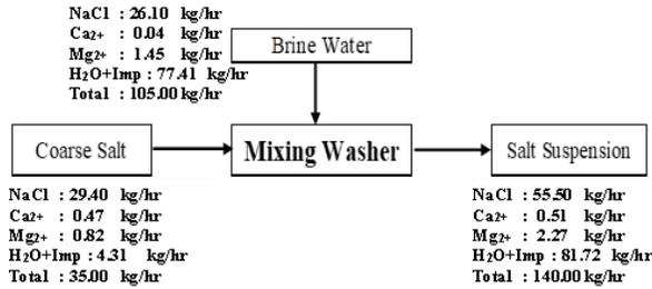
Fig. 1. Mixing Washer Mass Balance
