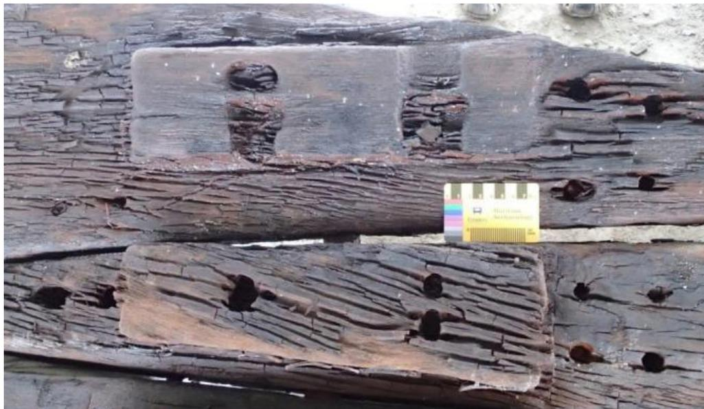
**Figure 15.** Deformation of a Lug (upper), After Long Exposure to Coastal Weather
