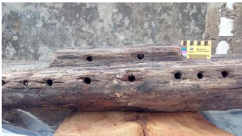
**Figure 12.** The Seam of the Keel Plank, Showing Holes for Ropes and Treenails
