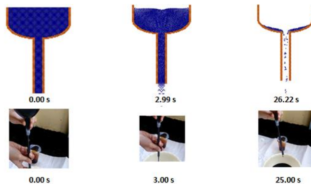
Figure. 6. Comparison of time of oil flow between simulation and experiment.
