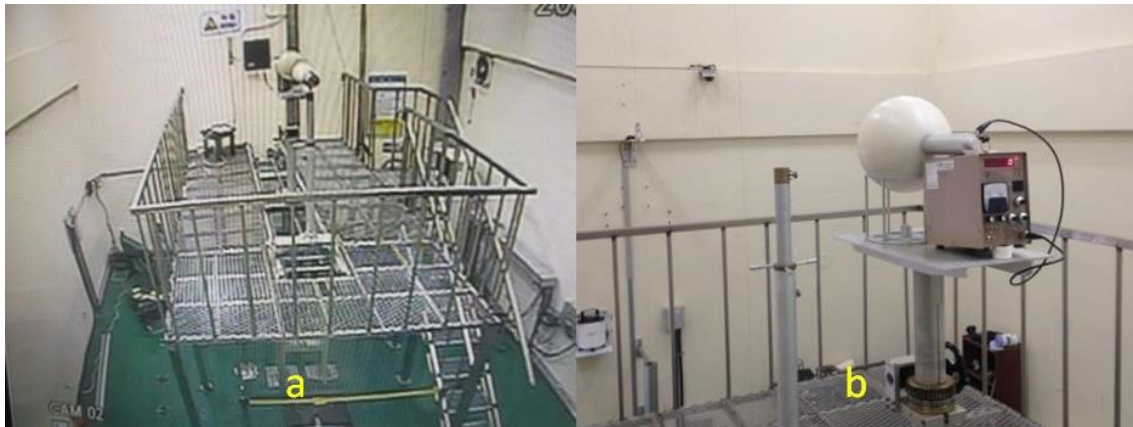
Figure 12. (a) KRISS neutron calibration room, and (b) measurement of ^{252}\text{Cf} neutron spectra using BSS
