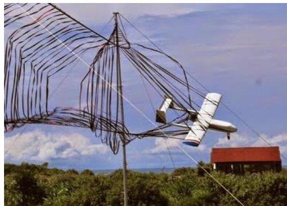
Figure 1-2. Aircraft recovery by using nets. (Pustekbang LAPAN, n.d.)
