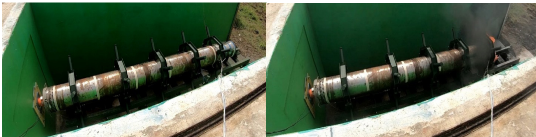
Figure 3- 5: Static test with C-shape adaptor, before and after burning.
