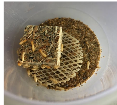
Gambar 3. Pengujian Rayap Figure 3. Termite testing
