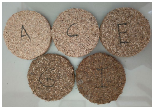
Gambar 5. Contoh Uji Redam Suara Figure 5 Sound Attenuation test sample
