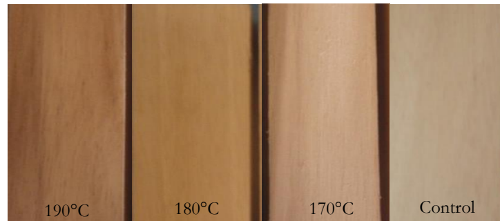
Figure 2. Surface performance of control and densified JUN wood at 170°C, 180°C, and 190°C compression temperatures
