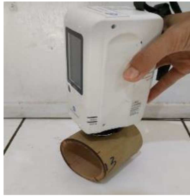
Gambar 4. Pengukuran warna batang bambu menggunakan colorimeter Figure 4. Measurement of bamboo culm's color using colorymeter
