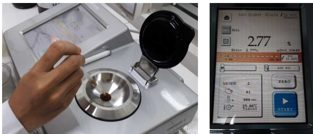
Gambar 5. Analisis kadar gula menggunakan refraktometer Figure 5. Sugar content analysis by refractometer
