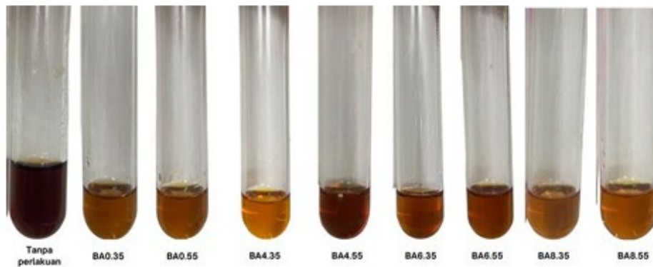
Gambar 6. Perbandingan minyak hasil organoleptik warna Figure 6. Oil comparison of organoleptic color analysis result
