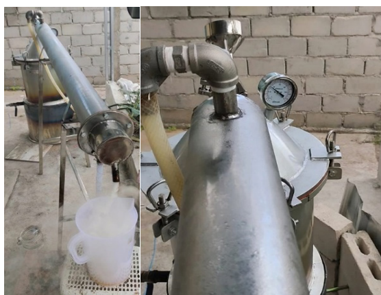
(Figure 1. Pyrolysis of Ulin Wood Waste Sawdust at 80°C for 8 Hours)
