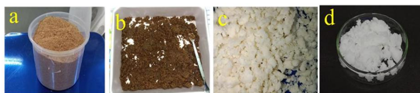
Figure 2. Stages of cellulose purification using the AHP-PAA bleaching sequence: (a) raw peel material, (b) delignified fibers, (c) intermediate AHP-treated cellulose, and (d) final PAA-Bleached cellulose
