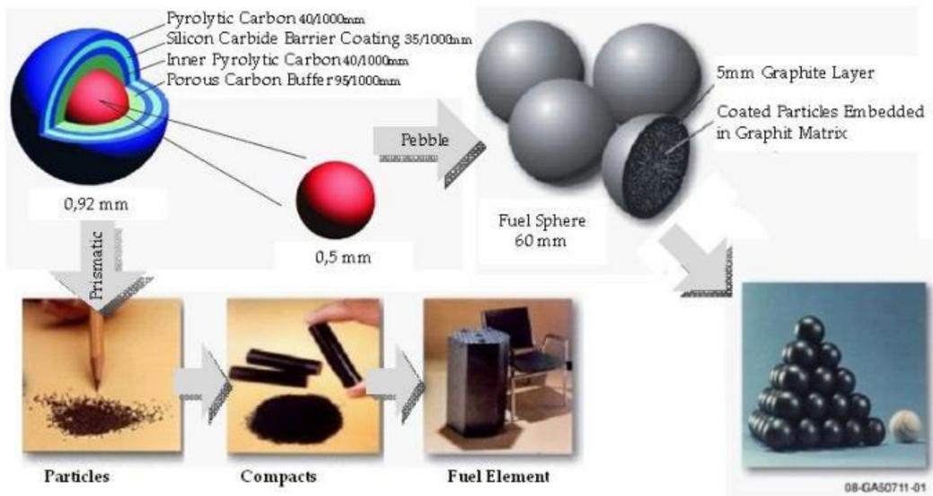
**Figure 1.** TRISO fuel particles for prismatic block-type and pebble bed-type cores [9]
