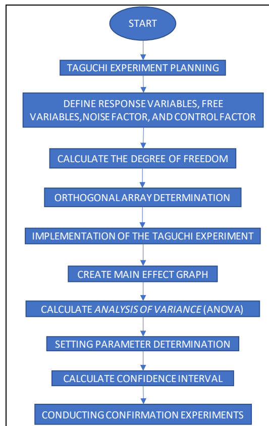
Figure 1. Design of experiment Taguchi method flow chart
