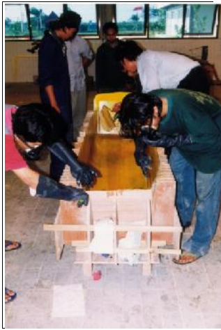
Gambar 43. Laminasi Model Test
