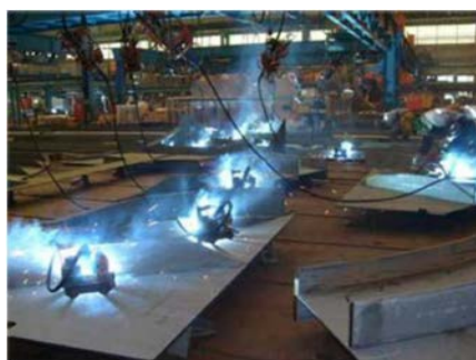
Gambar 2. Welding carriages in shipbuilding industry. (Sumber: Donghun Lee, 2014)
