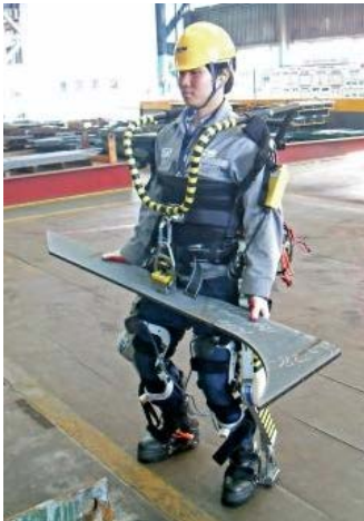
Gambar 10. Roboshipbulder , Image : Daewo shipbuilding (Sumber: techexplore.com ,2014)
