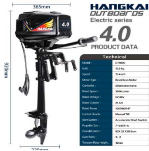
Figure 8. Ship engine specifications (Hangkai, n.d.)
