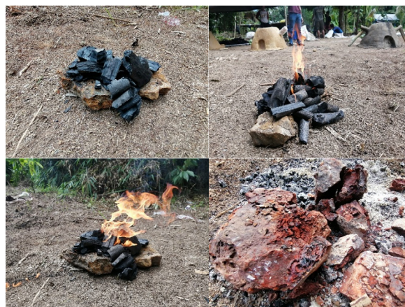
Figure 8. Experiment process roasting iron ore (Source: Author, 2019)
