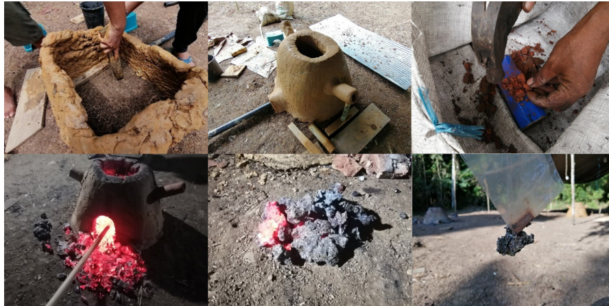
Figure 3. Experiment process furnace A (Source: Author, 2019)
