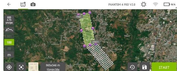
Figure 3. UAV flights path to cover the Contok River Basin, a sub-watershed of Garang River, Central Java Indonesia
