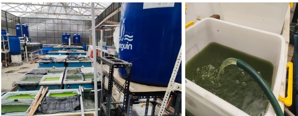
Figure 1. The installation of the recirculation system in experiment (a) and the filling of media/wastewater in (b).
