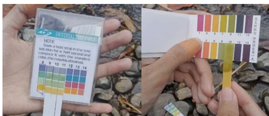
Figure 2. Measuring water pH at Ngablak Dengklek Dam using litmus paper for pH assessment.
