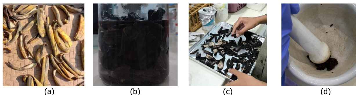
Figure 1. (a). raw materials before treatment, (b). After the carbonization process, (c). After the activation process, and (d) Powders used in the experiment.
