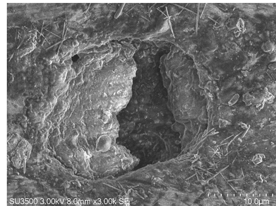
Figure 10. SEM results show that the porous size is estimated at 10 micrometers
