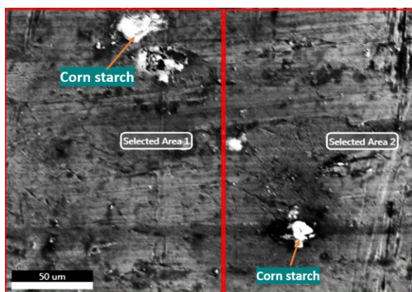
Figure 15. Selected area SEM EDS selected area 1 & selected area 2
