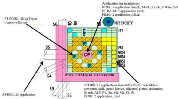
**Fig. 1.** Utilization of RSG-GAS, in the 100th core configuration
