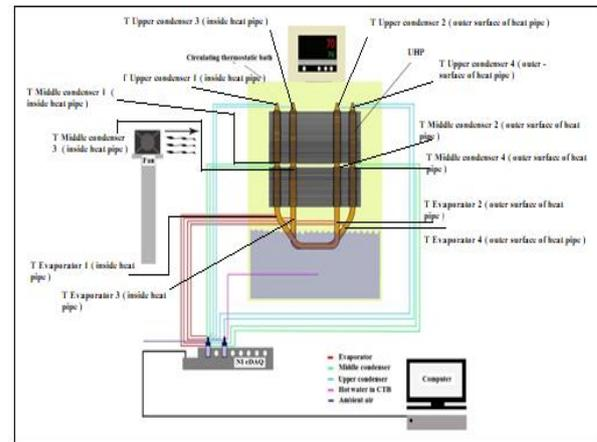
Fig. 1. UHP experimental setup[16]
