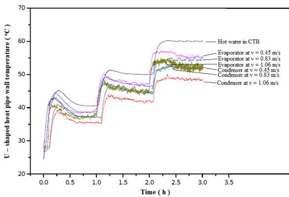
**Fig. 4.** The UHP wall temperature distribution at varied heat load and air coolant velocity
