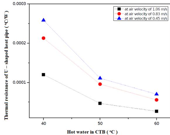
**Fig. 5.** The resistances of thermal of UHP[16]
