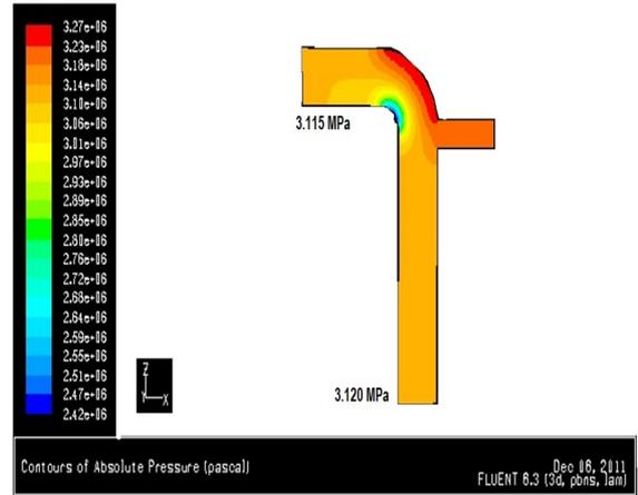
Fig. 5. Pressure contour at the inlet pressure of 3.120 MPa
