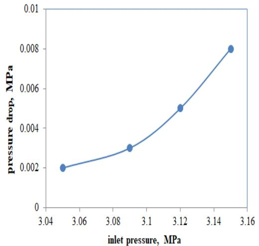
Fig. 7. The curve of inlet pressure vs. Pressure drop in outlet Pipe
