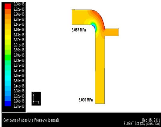
Fig. 4. Pressure contour at the inlet pressure of 3.090 MPa
