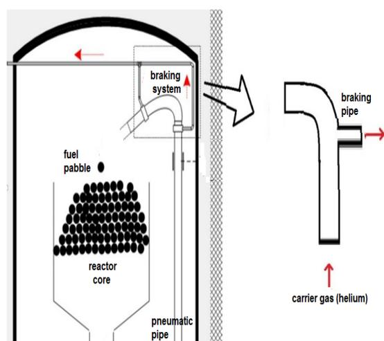
Fig. 2. Diagram of the braking system [9]
