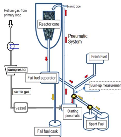
Fig. 1. Schematically Diagram of FHS Design [5]
