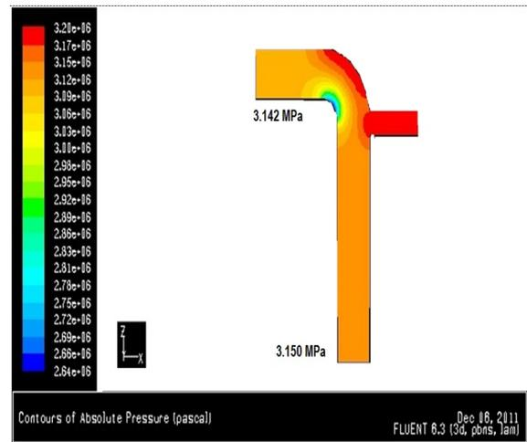
Fig. 6. Pressure contour at the inlet pressure of 3.150 MPa
