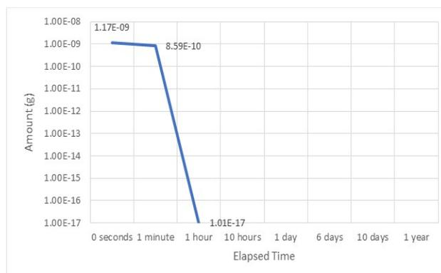
Fig 2. Amount of aluminum-28 produced from aluminum irradiation
