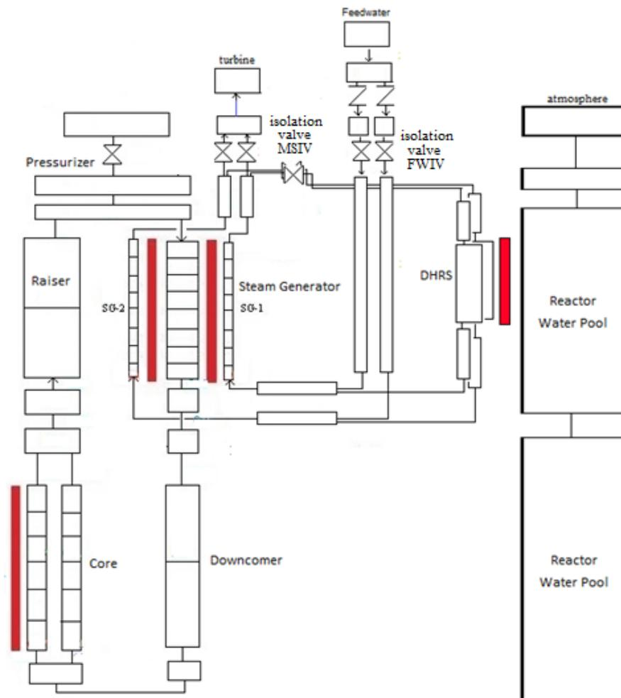
Figure 2. RELAP5 Nodalisation of NuScale Reactor System.
