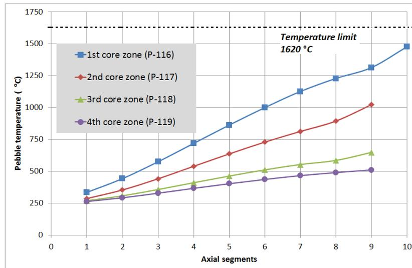
Figure 4. Pebble temperature distribution in the 4 core zones after adjustment in the middle core zone.
