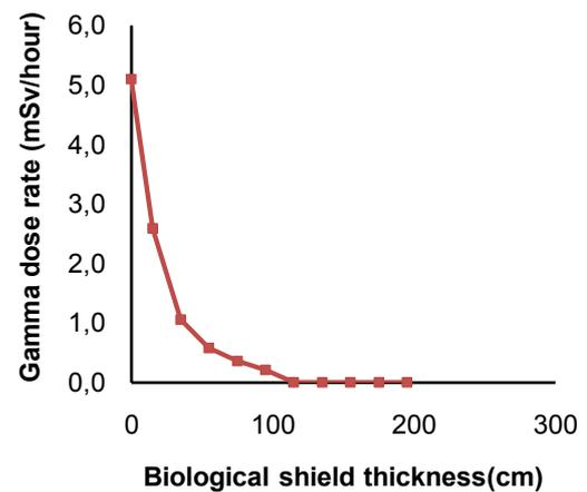
Figure 8. Relationship of gamma dose rate against shield the thickness of HTGR-10 MWth
