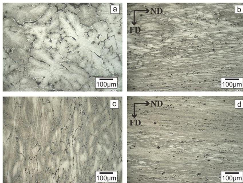
Figure 4. Comparison of Al-SiC microstructure pre and post forging. (a) Sample 1; (b) Sample 1-Forged; (c) Sample 2; (d) Sample 2-Forged. (ND for Normal Direction; FD for Forging Direction).
