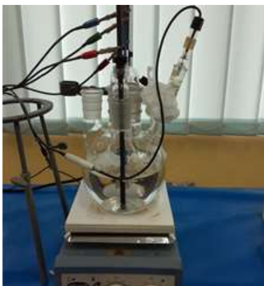
Figure 2. Cell circuit for corrosion rate measurement
