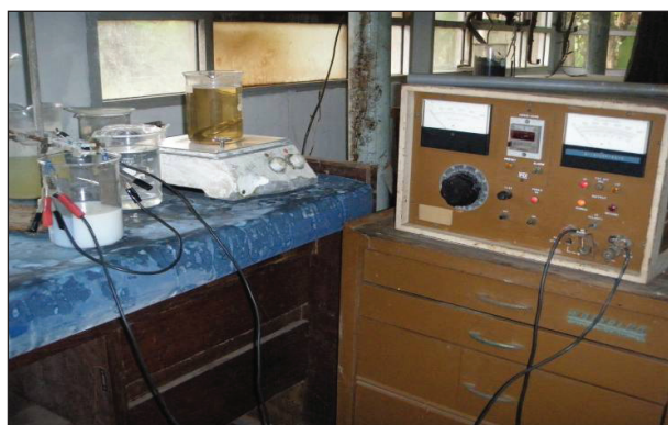
Gambar 4. Proses percobaan organic electrocoating
